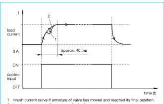
2 Inrush current curve if armature of valve has not moved.
